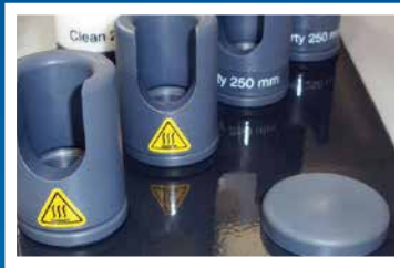
Timed System for pre-heating two endoscope supports at 38°.
