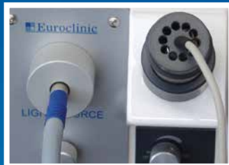
Neutral LED Light Sources (one or two channels), temperature from 4,100° K to 5,500° K. 180 Lumen — Storz connector for F.O. cable. Lamp life: Up to 50,000 hours (easy to replace).
